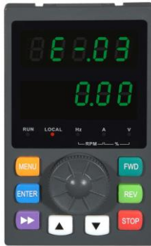
Fig. 4-5 Fault alarm display state
